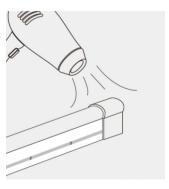
Dry the plug with hot wind or natural wind until make sure the installation is firm
