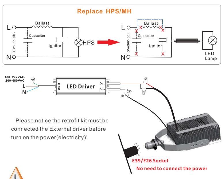
**N**Please remove any ballast or capacitor parts before doing the retrofit.
