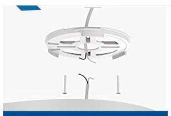
1: Fix the base plate onto the ceiling with 4 screws.
