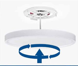
4: Install the ceiling lamp on the base plate by rotating clockwise.
