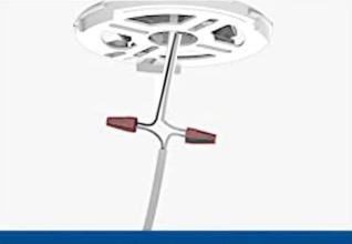
2: Connect L/N wires with quick connectors.
