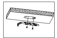
3.Attach the Canopy light with bracket by putting the ring on clips again. Connect the Black wire for line, white for Neutral, Yellow Green for Ground.
