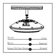
3. Screw the conduit into the hole on top of canopy light. Installation done.
