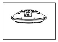
2.Fix the bracket on J-box ,and put the wire through the central hole for wiring
